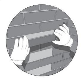
**5.3.** Check that surfaces of the tiles to be pasted are aligned exactly to the surface plane of pebbledash panels and are at the same height.
