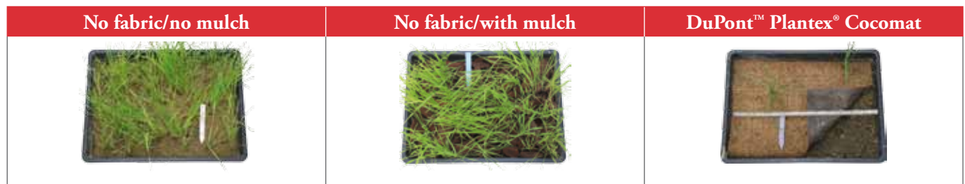
Germinated blackgrass seedlings through fabric after 5 weeks, Test result applied to a surface of 1m 2
