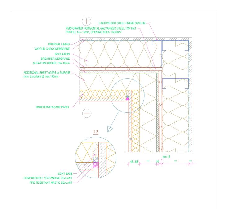
RAKETERM CLADDING SYSTEM WITH CAVITY
