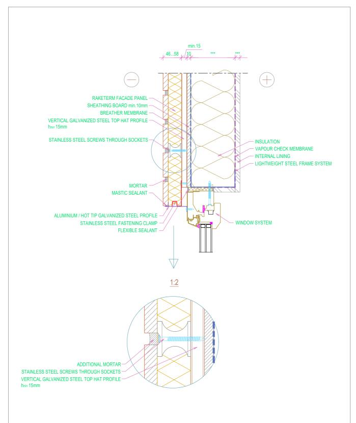
RAKETERM CLADDING SYSTEM WITH CAVITY VERTICAL STEEL FRAME WINDOW HEAD DETAIL WITH FLASHING
