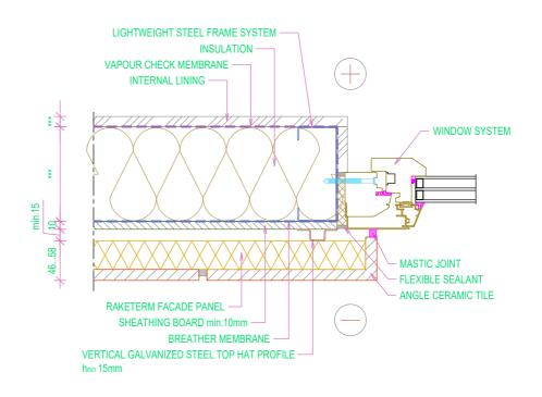
RAKETERM CLADDING SYSTEM WITH CAVITY
