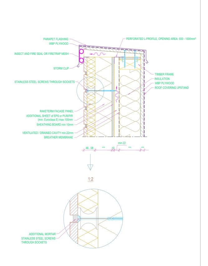
RAKETERM CLADDING SYSTEM WITH CAVITY
