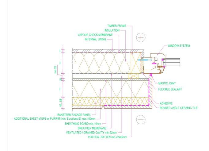
RAKETERM CLADDING SYSTEM WITH CAVITY
