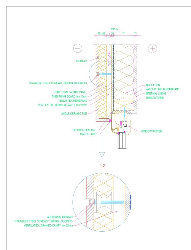
RAKETERM CLADDING SYSTEM WITH CAVITY
